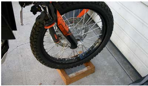
Block the front wheel securely
