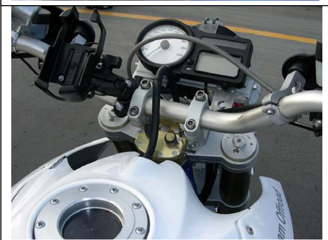
Correct tower pin height
