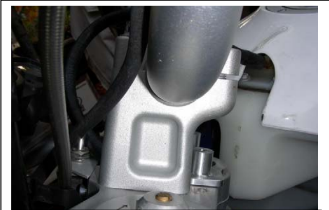
Correct lower perch position for this installation.
