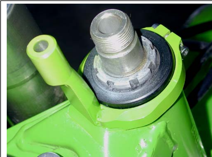
CR and KX share the same frame bracket for these years.
