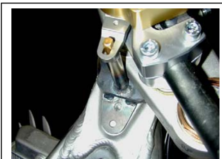
This shows just how close the stock triple clamp is to the vertical tower. Align so both sides are equal and yet the steering stops make contact.
