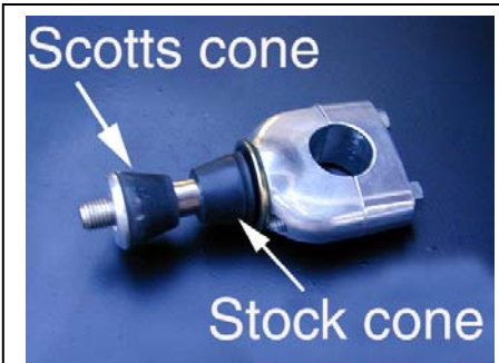
This shows the stock mounting perch
