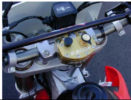
Stock handlebar cross bar are too close to the damper even in the reversed position mounting.
