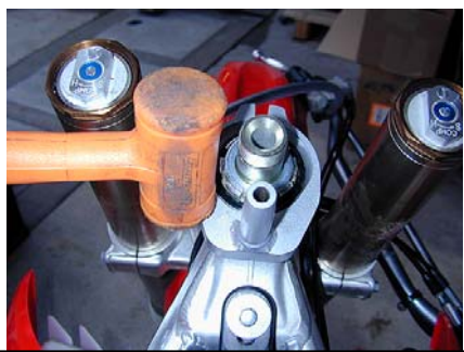
Tap & tighten, tap & tighten until the bracket is down flush all the way around the entire head tube.
