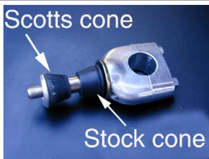
This shows the stock mounting perch
