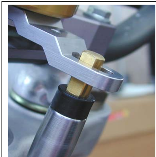
Best to have to the linkarm in the middle of the flats on the tower pin on this model.
