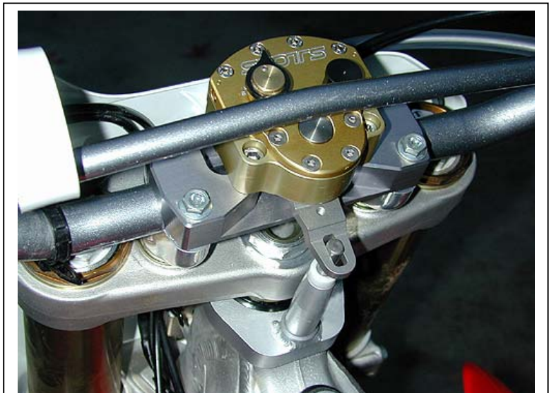
Finished kit using the stock bars with a bow in the crossbar.
