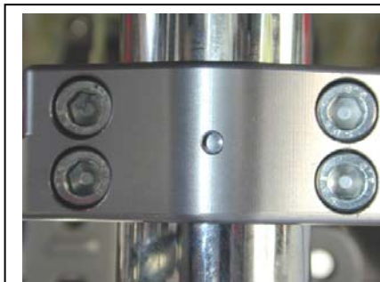
Shows the extra roll pin anchor point
