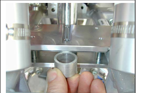
Spacer goes in between the frame plates
