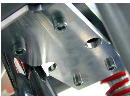
Bottom mount plate installed
