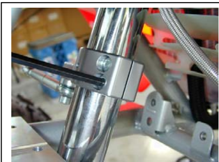
Temporarily install steer tube bracket
