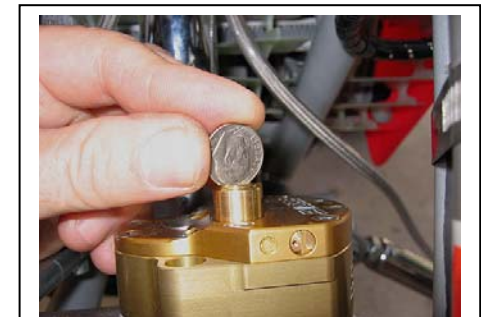
Adjusting the high speed with a dime
