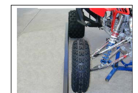
Aligning the tires straight ahead
