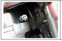
Key lock on XR650L may need slight filing in rare cases. This is under the stock triple clamp on the front side.
