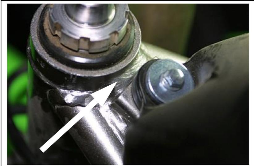
The welds vary considerably from bike to bike so be sure to file downward until the bracket fits properly retaining the head tube sizing
