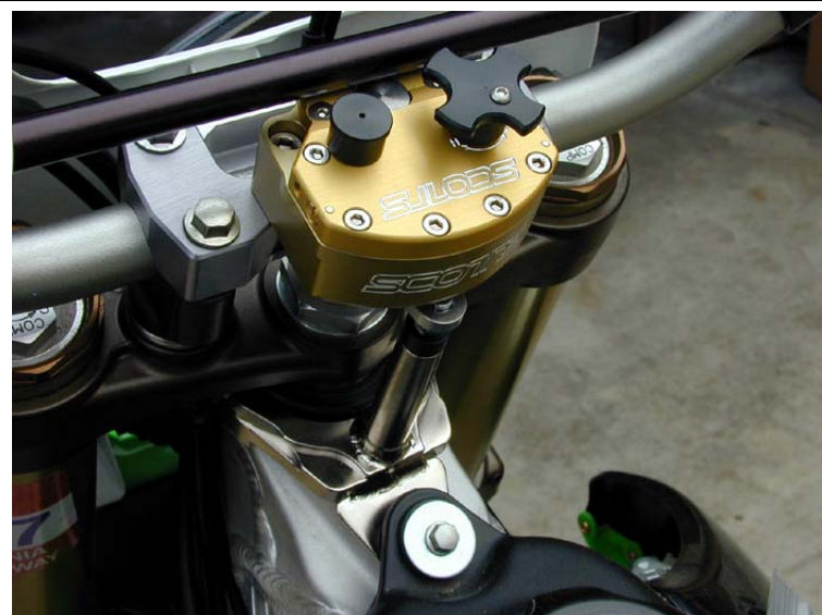
Shown here is the reverse mounted damper that is required when using the stock standard diameter bars. Large knob is optional.
