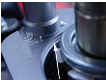
Be sure the frame bracket is all the way down flush with the head tube, all the way around the entire surface.
