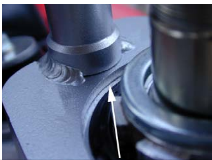
Be sure the frame bracket is all the way down flush with the head tube, all the way around the entire surface.
