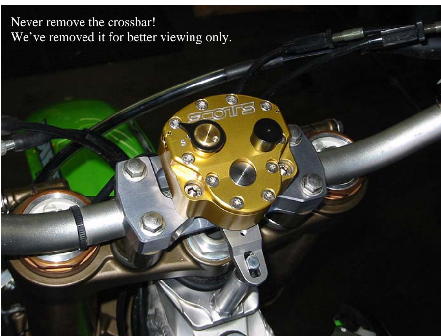
This shows the "spacer-washer" installed on top of the jam nut and under the triple clamp.
