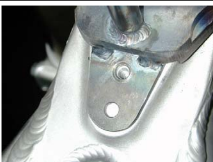
This shows the alignment of the frame bracket after the front pinch bolt has been properly tightened. The forward hole is for the X models and the rear hole fits the CRF250R models.
