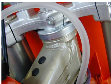
This needs very little filing at the weld
