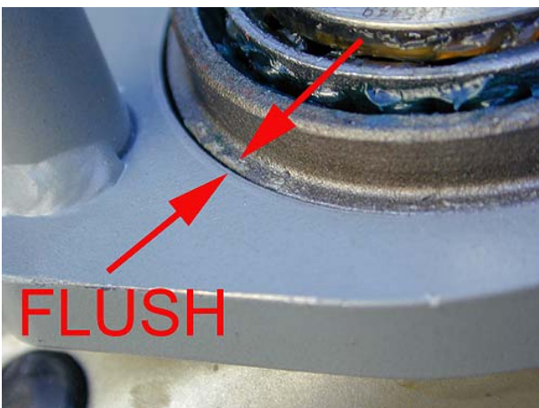
File the welds so the groove shows all the way
