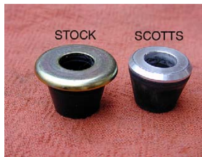
Our replacement cone goes on the bottom And butt the nut directly against the cone.
