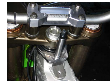
Our replacement cone goes on the bottom And butt the nut directly against the cone.
