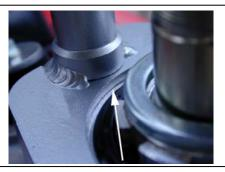
Be sure the frame bracket is <u>all the</u> <u>way down</u> flush with the head tube, all the way around the entire surface.
