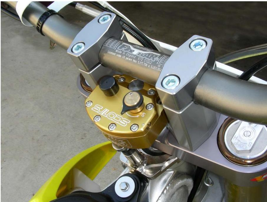
Finished SUB Mount shown with the Scotts Solid Mounted Triple Clamp
