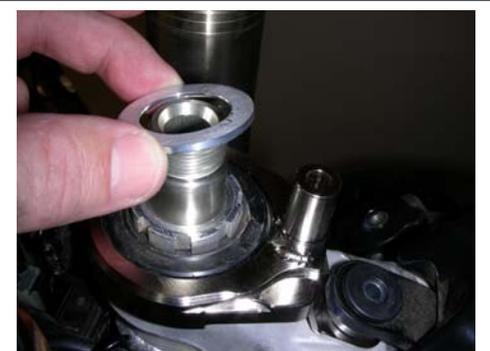
Some models, not all, may require this stem spacer to give more clearance between triple clamp and frame bracket.
