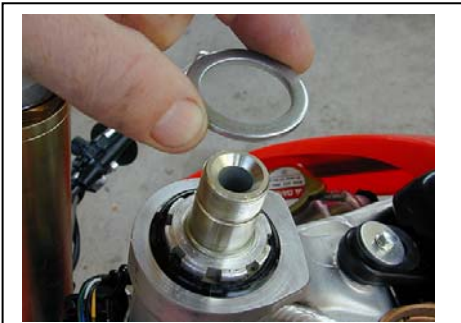
Install special .125" washer supplied
