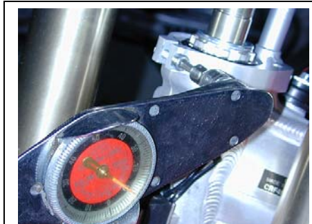
Torque the frame bracket pinch bolt to at least 96-108 inch lbs., or the equivalent of 8-9 foot lbs.
