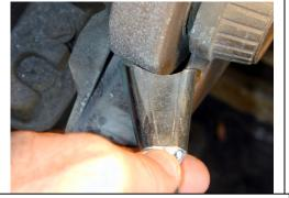
Grinding the base to match frame shape
