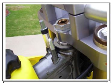
Weld on tower in place after welding
