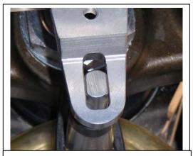
Try to center the pin in the linkarm slot, use welding rod on each side to hold in place.
