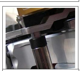
Tower Pin flush as shown, or above top of linkarm by 2mm with rubber mounts.
