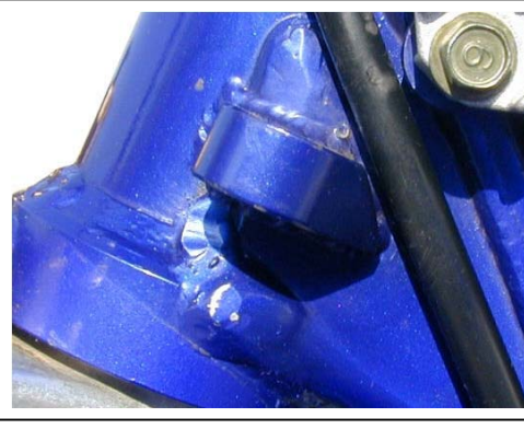
Be sure the Lug bolt head clears the stock steering stop on the lower triple clamp.
