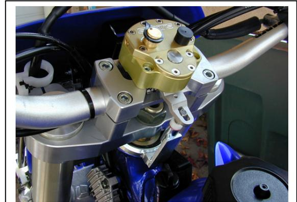
Shown above are the Scotts Billet Triple clamp with Protaper bars. These require no modifications and bolt right on.
