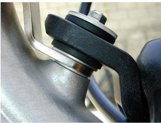
Spacer/washer is under the frame bracket tab
