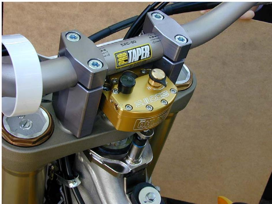
Shown is the YZF stock triple clamps, with Scotts SUB mount installed.
