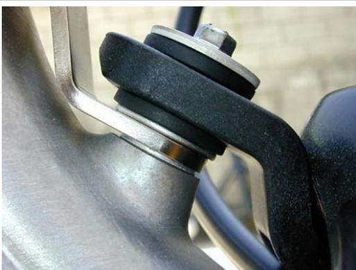
Spacer/washer is under the frame bracket tab
