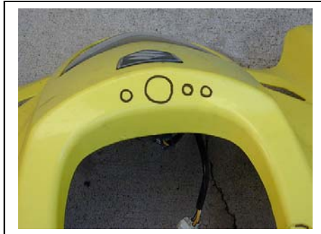
Marking where the gauges will go
