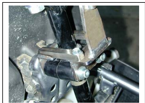
Frame bracket installed
