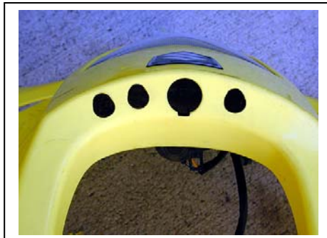
Finished gauge holes
