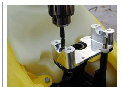
Drilling the 8mm holes
