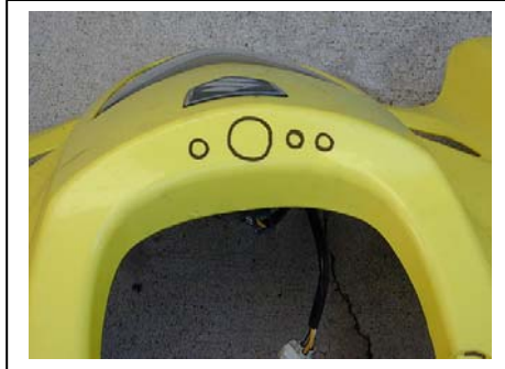
Marking where the gauges will go
