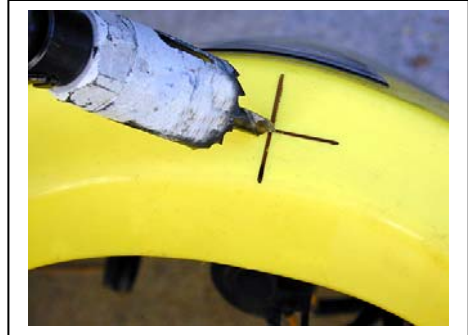
Drilling 1" hole for the ignition
