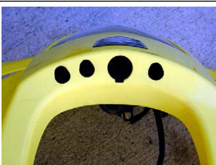
Finished gauge holes
