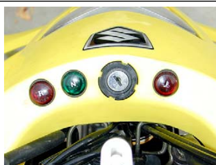
Finished gauge relocation
