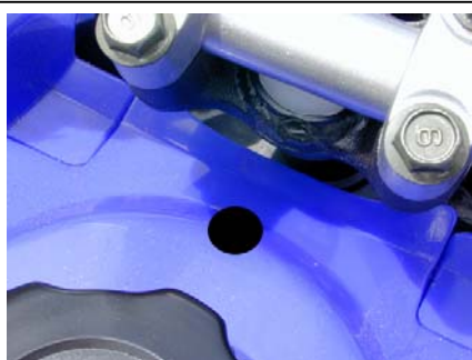
Finished hole for the tower post
