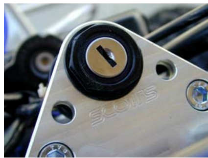
Key switch installed in new bracket
