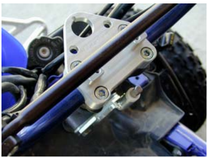
Barclamp & frame bracket installed
