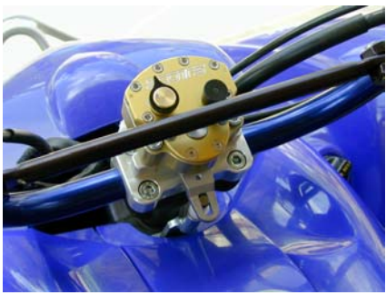
Finished "Standard" Mount kit position when using no key or relocating the key
