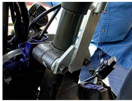
Frame bracket installed correctly with the star locking washer in between the frame bracket and pillow block
