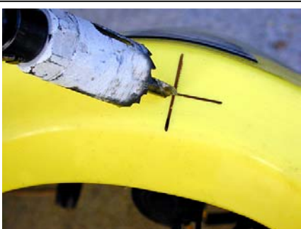
Drilling 1" hole for the ignition
