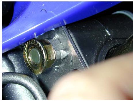
Butting the spacer nut against the stocker
