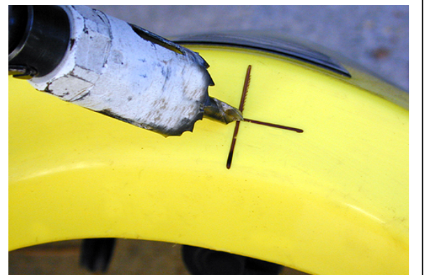
Marking and drilling the light relocation holes.
