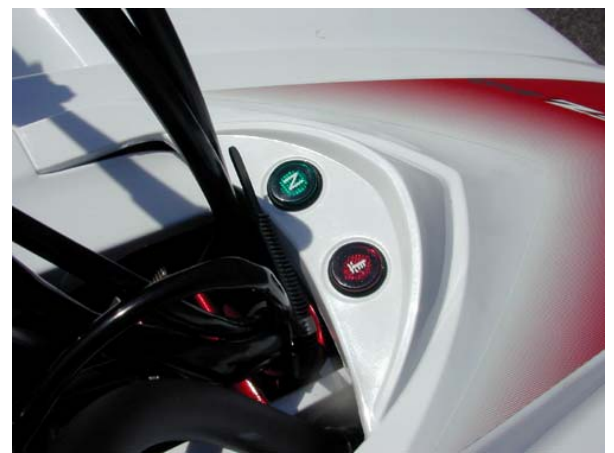
Relocate the lights to the front shroud like the YZF, or eliminate the lights all together.
