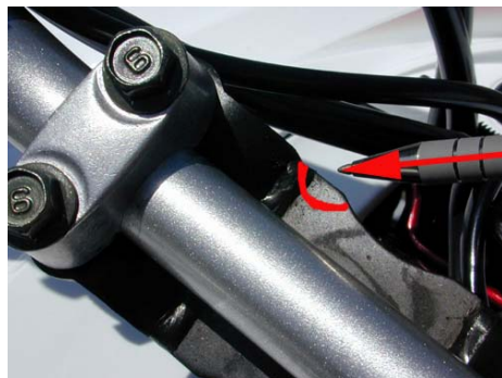
Possible grinding required here
