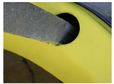
Notching the ignition hole with file
