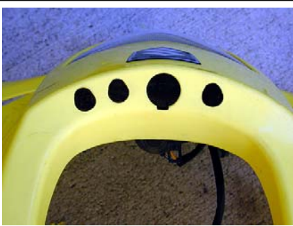
Finished gauge holes
