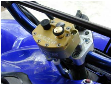
Finished Reversed mounted kit should look like this utilizing the key switch in our handlebar clamps.
