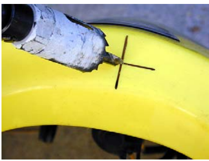
Drilling 1" hole for the ignition
