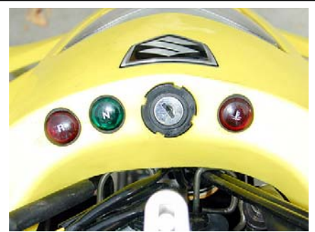
Finished gauge relocation
