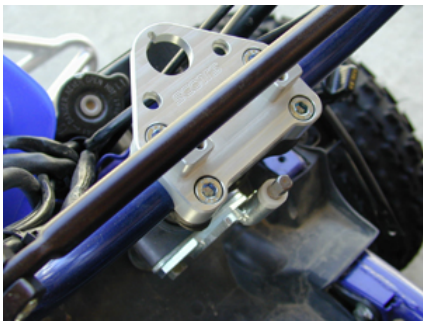
Barclamp & frame bracket installed
