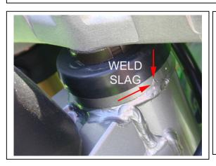
Weld slag or any obstructions that would prevent the frame bracket from clamping tightly and securely to the head tube, must be removed before bracket is installed if you expect it to stay on. Simply file it away while trying to retain a concentric diameter.
