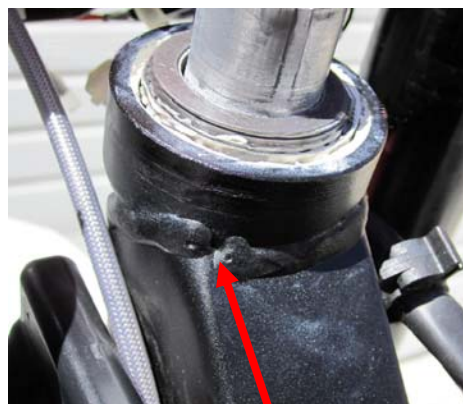
File welds keeping the frame bracket from clamping tightly around head tube
