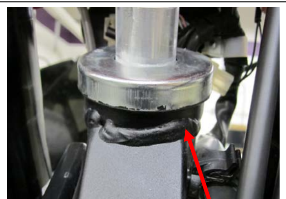
File welds keeping the frame bracket from clamping tightly around head tube
