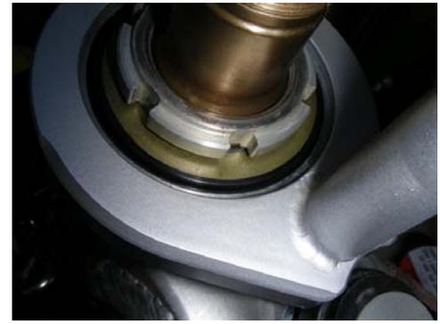
The frame bracket must be flush, all the way around on the top of the head tube.
