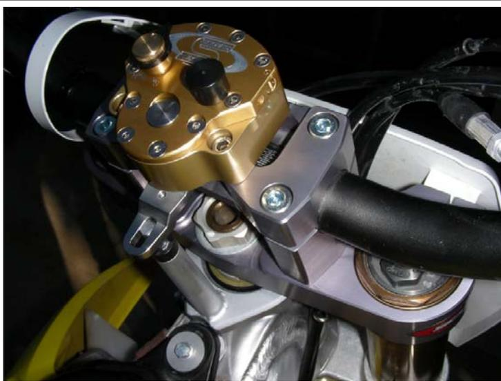
Finished kit with the Scotts Solid Mounted Triple Clamp
