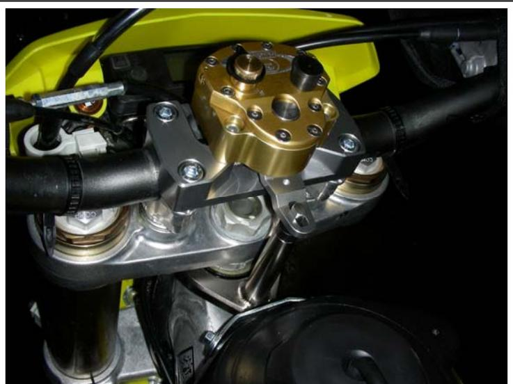
Finished kit using the stock triple clamps and oversized tank
