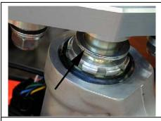
Install the spacer here, below the triple clamp and on top of the bearing nut.
