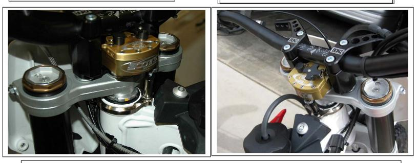
The Black Sub mount is this photo is only to help pronounce the part for the photo and installation ease. The actual Scotts Sub Mount is normally Titanium in color. (The large black knob shown is an extra option).
