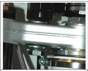
Note the bolt head to frame bracket clearance
