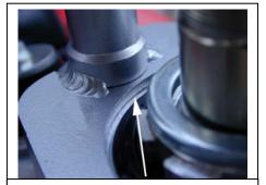
Be sure the frame bracket is <u>all the</u> <u>way down</u> flush with the head tube, all the way around the entire surface.
