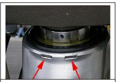
The frame bracket must "dig" into the back of the head tube if you expect it to stay on. This does NOT jeopardize the bearing.
