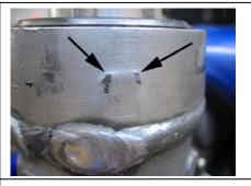
Clean the head tube of casting bumps
