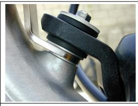
Spacer/washer is under the frame bracket tab
