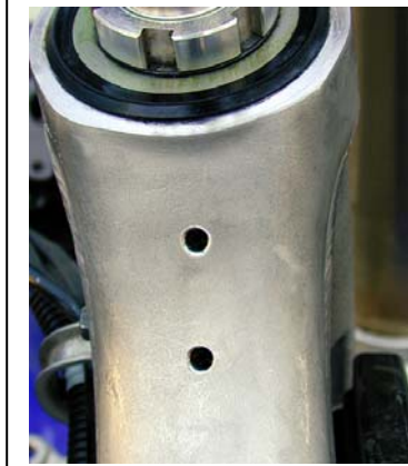
Be sure the frame bracket is all the way down flush with the head tube, all the way around the entire surface.
