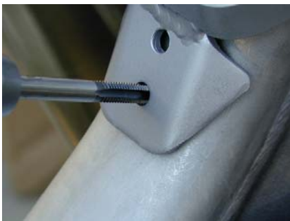
Drilling and tapping one hole at a time. Keep the drill and tap perpendicular to the bracket tab surface.
