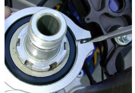
Spread the frame bracket gently and slide it on in one clean motion.
