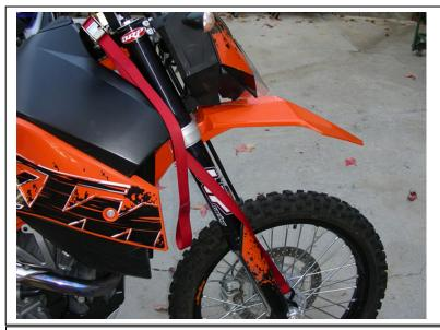
OR: Hook a tie down on the front axle, then up and over the back bone and back down to the other side axle or to the opposite side lower triple clamp to secure the forks in place. This is very important as the forks can roll away from the bike once the triple clamp is off.
