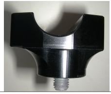
Front of bike is at the left in this picture. This shows the lower Barclamp in the Forward position, centerline of bars are in front of the centerline of bolt.
