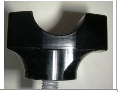
Front of bike is at the left in this picture. This shows the lower Barclamp in the rearward position, centerline of bars are behind the centerline of bolt.
