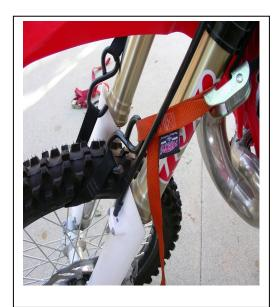
Run a tie down through the front wheel, up and over the back bone to secure the forks in place. This is very important as the forks can roll away from the bike once the triple clamp is off.
