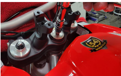
Remove the main triple clamp nut with a 12mm allen socket.
