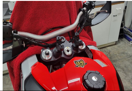
Remove handlebars and lay forward in a towel or protective blanket
