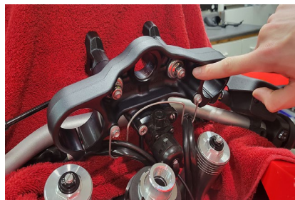
Loosen the 15mm perch nuts on the bottom of the triple clamp.
