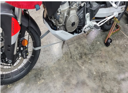
Tie the front wheel to the foot pegs using a tie down.
