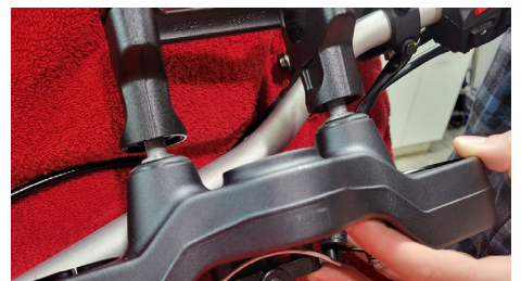
As you Loosen the 15mm perch nuts, the perches un-thread and rise upward and off. Un-do each side a little at a time.
