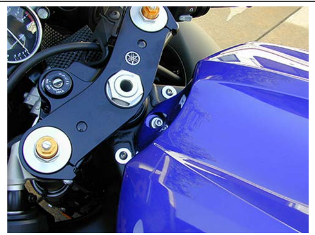
This photo shows the bike with the stabilizer kit removed and the holes plugged. We left them silver in the photo to show you how it looks, although the bolts and washers could be black to blend with the frame OR optional black plastic plugs like the ones Yamaha uses on the top of the triple clamp could be used as well.
