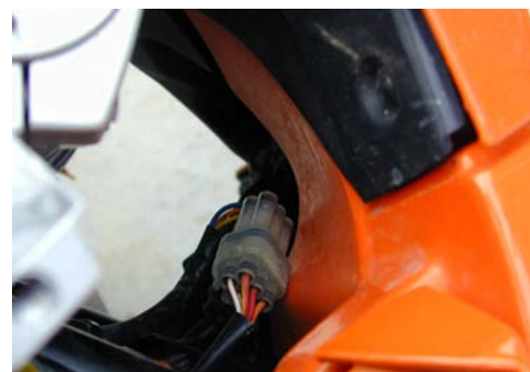
Locate and unplug ignition switch right side
