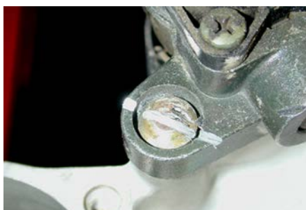
Cut a slot in the head for a screwdriver
