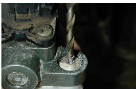
Drill a hole dead center for an easy out or..
