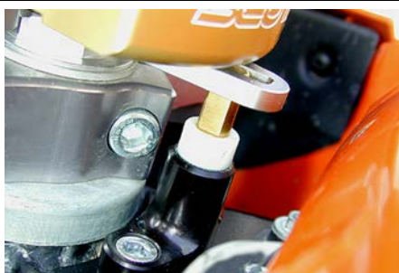
Frame bracket installed-note tower pin height
