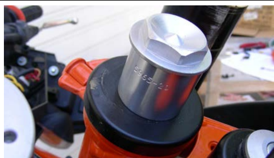
Tool to hold forks on while working with TC off.
