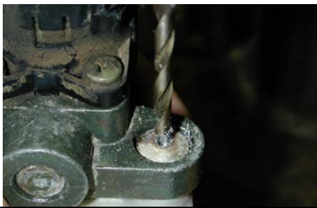
Drill a hole dead center for an easy out or..
