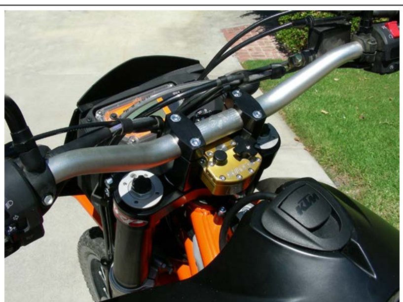
This shows the first generation mount which has been upgraded now to a rubber sub mount for better vibration absorption (see left photo). The large knob pictured in this photo is an optional part.
