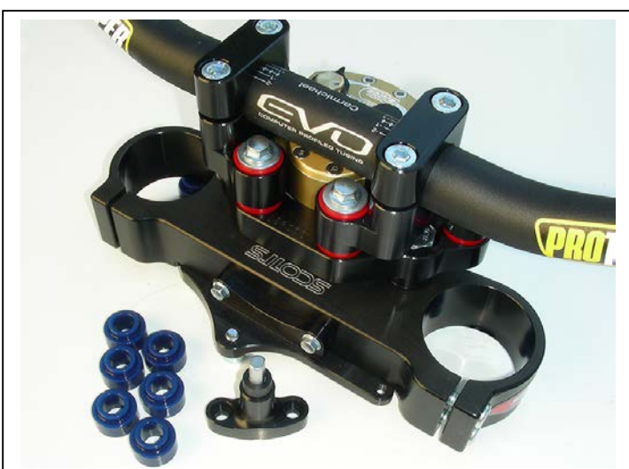
This shows the newest generation RSA, rubber sub assembly to reduce vibration and fatigue even more than before. We supply an extra set of different density rubber cones to help each user customize their particular desired feel.
