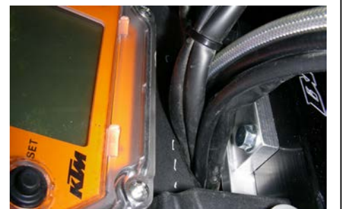
Cables routed properly, no binding
