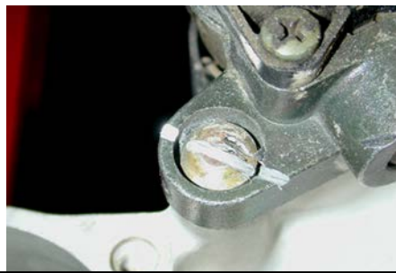
Or Cut a slot in the head for screwdriver
