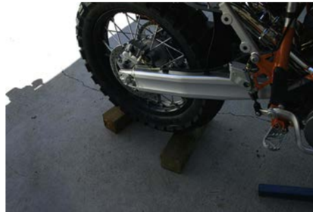
Block up the rear to put pressure on front
