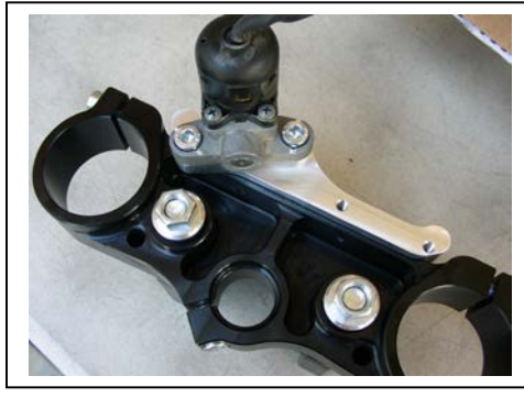
Key switch mounted to underside
