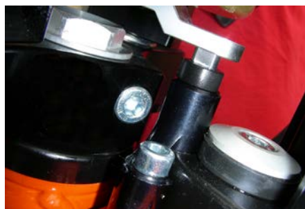
Frame bracket installed-note tower pin height
