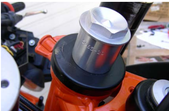
Tool to hold forks on while working with TC off.
