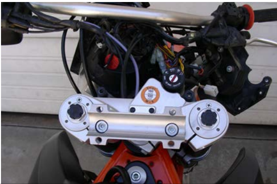
Roll the bars up out of the way and tie up.
