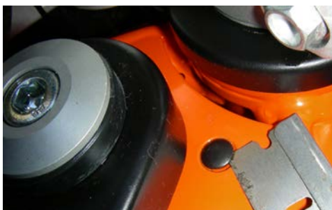
Frame bracket hole, remove plastic covers
