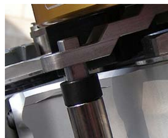
Tower Pin correct height
