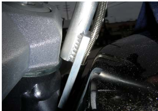
Move the weld on tower around to find best spot.
