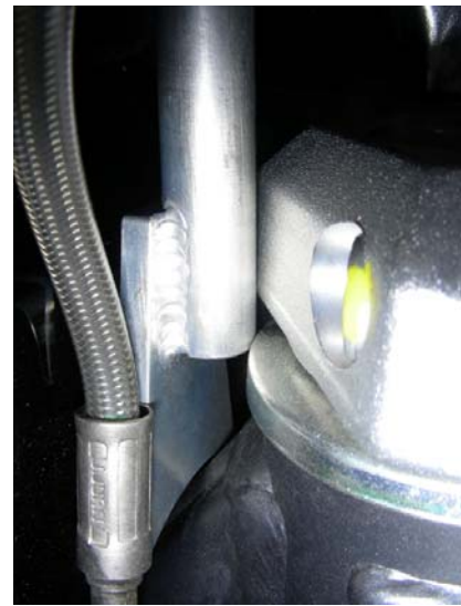
This shows the tower clearing the bearing cover, triple clamp at full lock, brake cable clearance and tank
