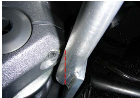
May need trimming here to clear triple clamp
