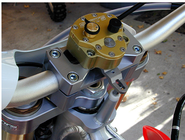
Above photo shows the billet Scotts Triple clamp and Oversize bars, available as a kit from Scotts Performance.
