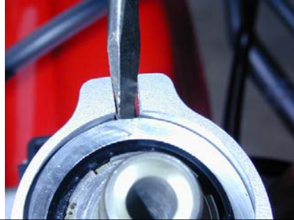
Remove bolt & spread bracket to install
