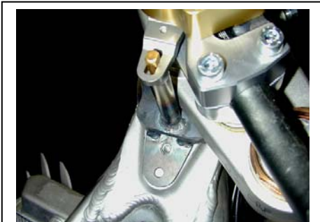
This shows just how close the stock triple clamp is to the vertical tower. Align so both sides are equal and yet the steering stops still make contact.
