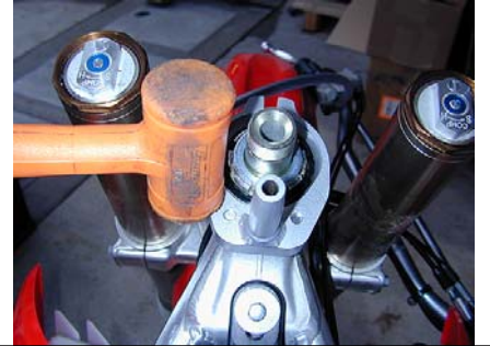
Tap bracket down until securely flush
