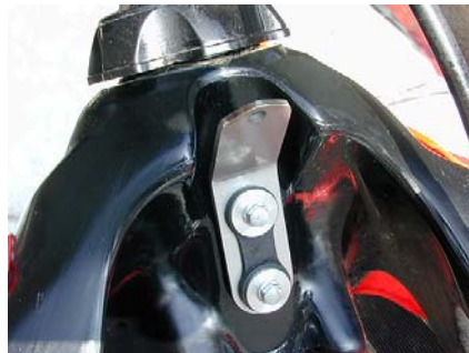
This shows the replacement X tank bracket that goes on top of the frame bracket tab.
