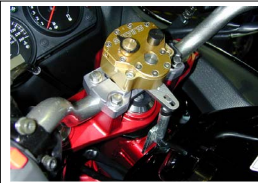
Align the linkarm and tower pin so the pin is in the middle of the slot.
