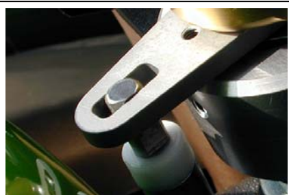
Align the linkarm and tower pin so the pin is in the middle of the slot.
