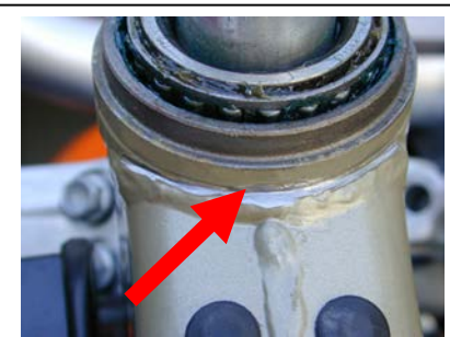
File any welds so the groove shows all the way around.
