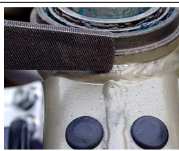
Using a sharp file, start at the high spots and trial fit the bracket until it fits.
