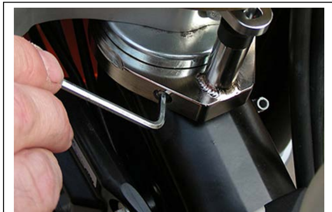
Use BLUE loc-tite (not red) on the set screws.
