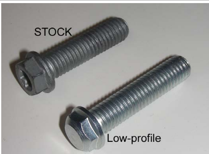
Shown here is the stock and new low profile bolt for the triple clamp pinch bolt on bikes with little or no clearance.
