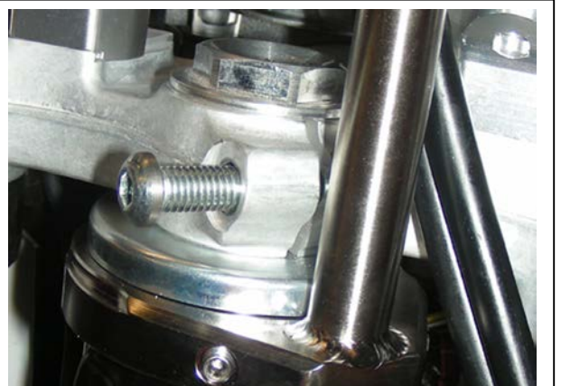
Install the special low profile bolt to gain more clearance as the triple clamp swings past the tower.
