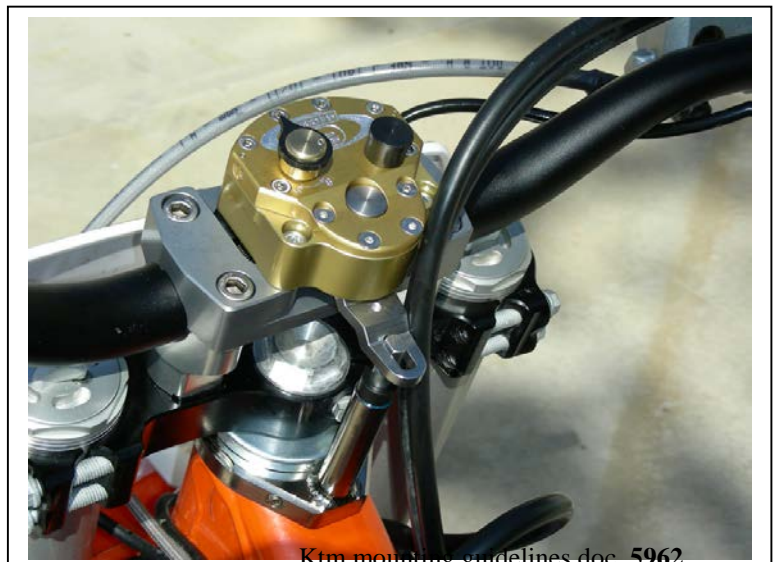
Install the special low profile bolt to gain more clearance as the triple clamp swings past the tower.
