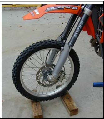
Block the front wheel & forks
