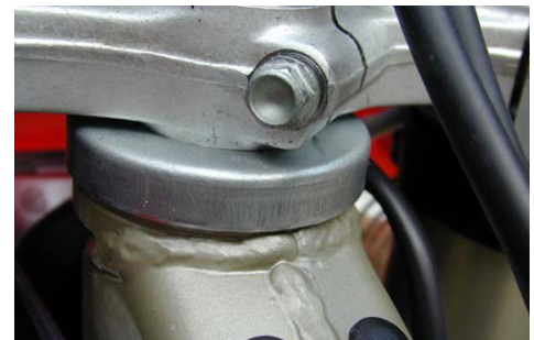
This will need a lot of filing at the weld
