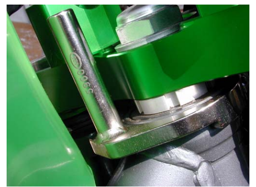
Photo shows frame bracket flush on top side
