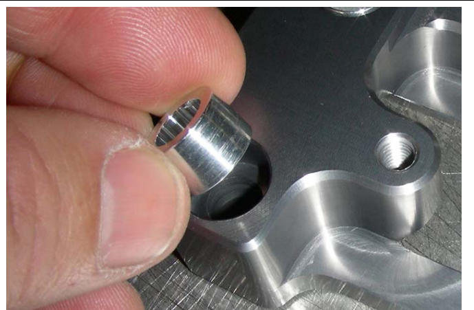
DRZ-SM models need the bushing in one hole for key switch
