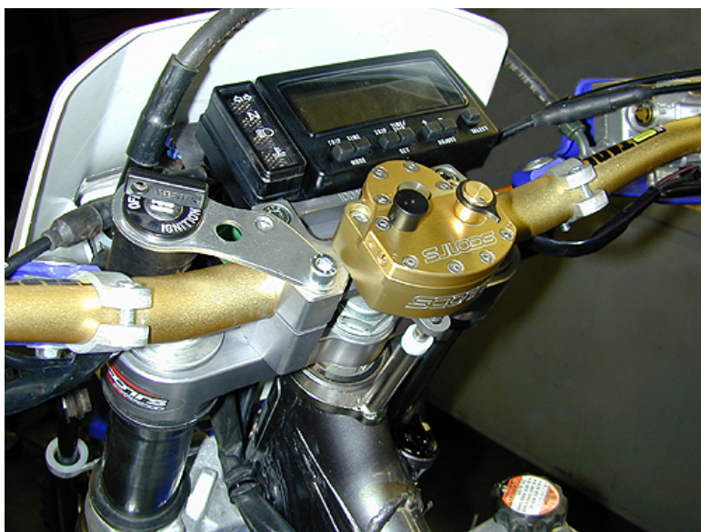
This shows the key switch mounted to the rear barclamp hole and the stabilizer in the "Reversed" mounting position, to clear the gauges.
