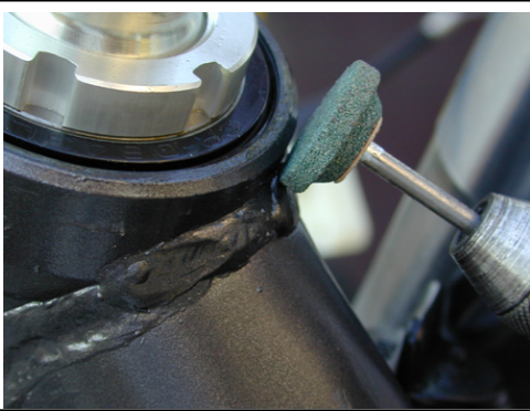
Optional way to remove weld be careful not to grind on head tube itself
