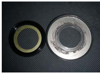
New seal on the left. Stock seal on the right. Must use new seal with our kit to allow frame bracket to fit.
