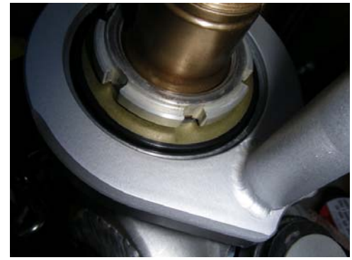
The frame bracket must down flush, all the way around on the top of the head tube.
