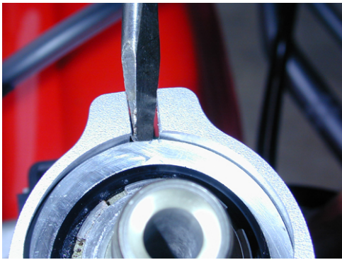
Spread the bracket gently, only enough to allow it to slide over the head tube.
