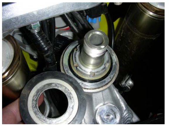
New seal on the left. Stock seal on the right. Must use new seal with our kit to allow frame bracket to fit.
