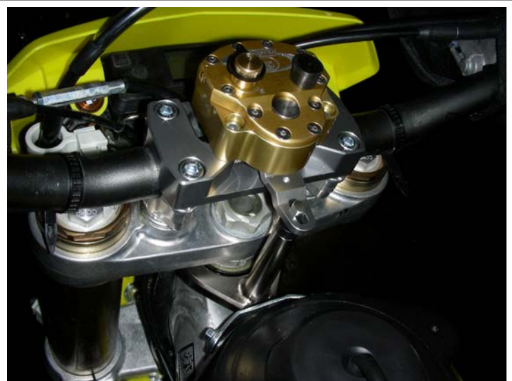
Finished kit using the stock triple clamps and oversize tank
