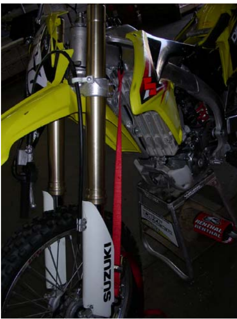
Be sure to tie the forks to the frame as it's very easy for them to roll away from the bike once the jam nut is released on the stem.
