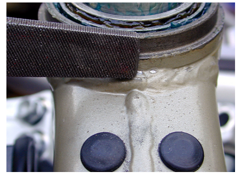
Using a sharp file, start at the high spots and trial fit the bracket until it fits.
