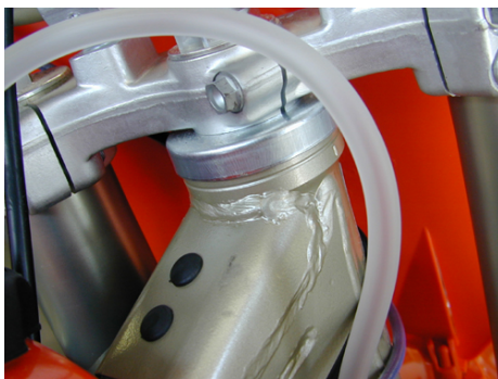
This example needs very little filing at the weld
