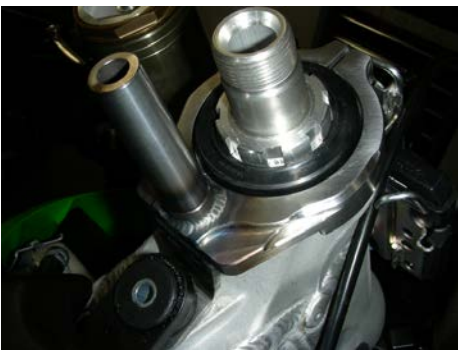
Be sure the frame bracket is all the way down flush with the head tube, all the way around the entire surface.
