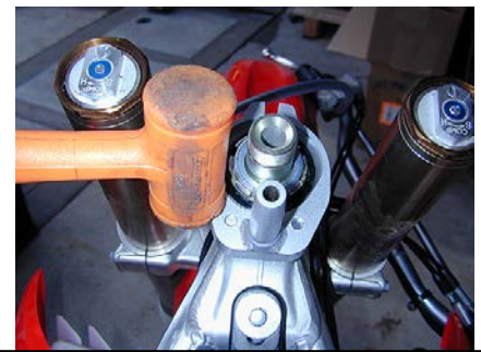
Tap bracket down until securely flush
