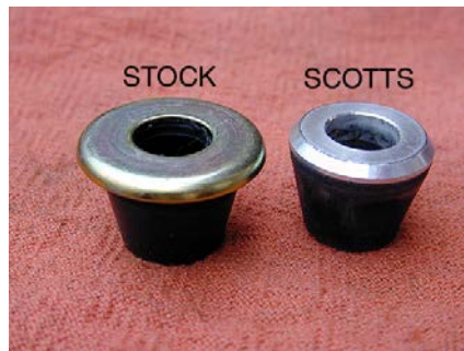
Our replacement cone goes on the bottom And butt the nut directly against the cone.
