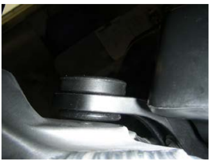
250 only: Invert the tank bushing
