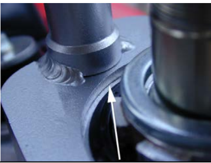
Be sure the frame bracket is all the way down flush with the head tube, all the way around the entire surface.
