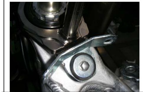
IMS tank bracket installation
