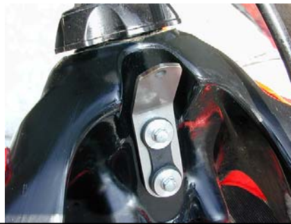
This shows the replacement X tank bracket that goes on top of the frame bracket tab.
