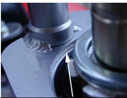
Be sure the frame bracket is all the way down flush with the head tube, all the way around the entire surface.
