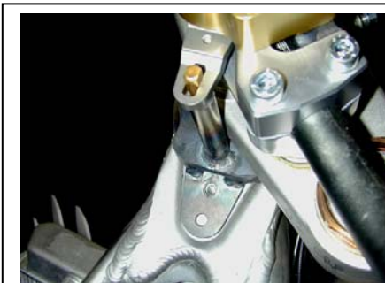
This shows just how close the stock triple clamp is to the vertical tower. Align so both sides are equal and yet the steering stops still make contact.
