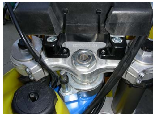
Note how the stabilizer bolt-holes are aligned over the steer tube center
