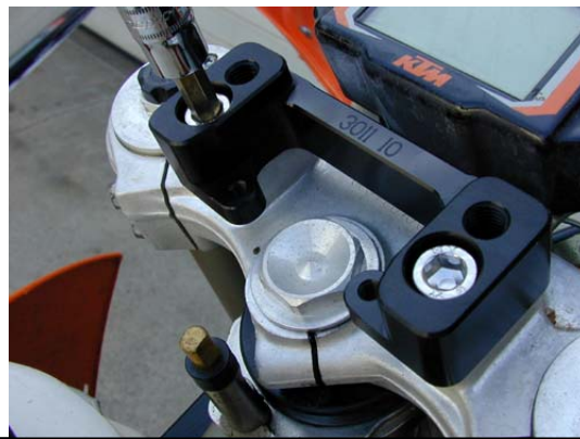
Note how the stabilizer bolt-holes are aligned over the steer tube center
